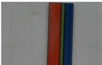
Simple template 6mm wide set up with the 60:40 split plus tolerance. Operator laid pack against this template. “Inside” green zone was a pass.
